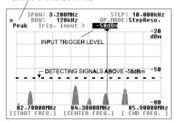
WHILE NO SIGNAL ABOVE THE TRIGGER LEVEL IS DETECTED [Trig. wait...] IS DISPLAYED
