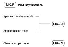
When the continuous peak detection is being used in the channel scope mode, the marker will automatically move to the strongest signal detected in the process of sweep. Press the **MK.F** key to automatically tune the companion receiver to the strongest signal instantly, so that you can monitor the active frequency.
