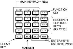
The **FUNC** key enables activation of the second function keys. When pressed the '**FUNC**' legend appears in the top left corner of the LCD in reverse contrast YELLOW text.
