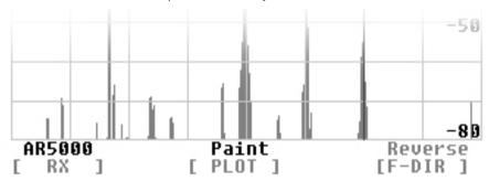
The box where the type of receiver is shown will be in reverse contrast. Rotate the main dial to scroll through applicable receivers one after another. Press the **ENT** key (**kHz** key) to determine the companion receiver. There are no other features of the RX configuration menu.
