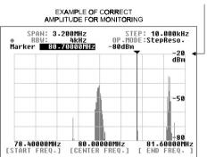
Effective use of the attenuator of the companion receiver will be required to prevent saturation of received signal particularly when an external aerial is used.
