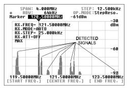
THIS EXAMPLE SHOWS THE RESULT HAVING MONITORED THE VHE AIRBAND WITH THE MAX HOLD MODE. IT IS POSSIBLE TO ANALYZE THE DETECTED SIGNALS AFTER THE SWEEP HAS FINISHED
